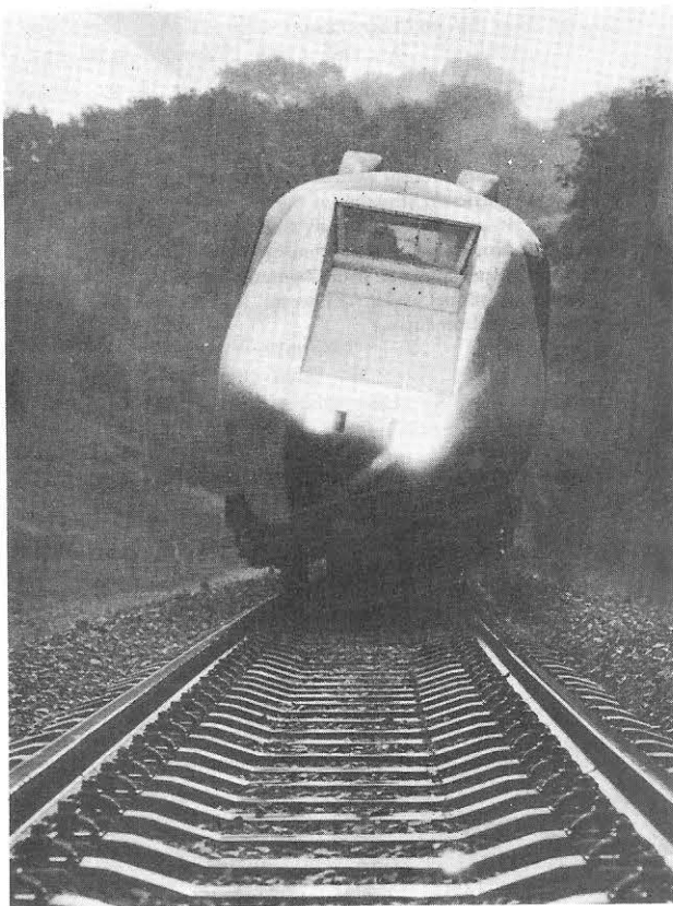
Fig. 9: APT-E rounds the 1.15 km radius Upper Broughton curve on the test track at 195 km/h (12° cant deficiency) whilst lateral track forces and displacements are measured
